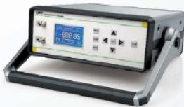
The DPC measures and generates pressures and consequently it is more than a mere measuring instrument - it can also be applied as test and calibration instrument for pressure sensors and pressure switches. Thanks to internal pressure generation no auxiliary tools are required for operation. An internal Li-ion battery is available for mobile operation. Parallel operation of mains and battery supply allows for maximum flexibility.
